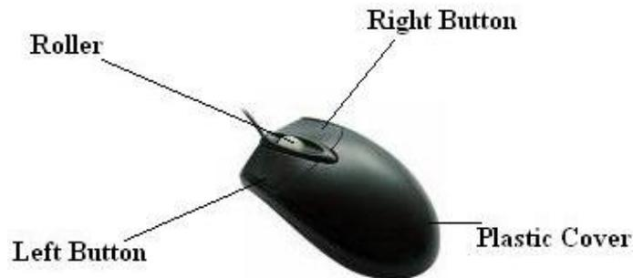
Its name is derived from its shape, which looks a bit like a mouse, with its connecting wire that one can imagine to be the mouse's tail. A Mouse rolls on a small ball and has two or three buttons on the top. When you roll the mouse across a flat surface on the screen, sensors sense the mouse in the direction of mouse movement. The cursor moves very fast with a mouse giving you more freedom to work in any direction. It is easier and faster to move through a mouse compared to movement using keys.
