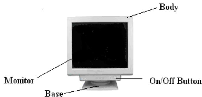
In CRT monitors, the image is projected on the screen by directing the electron beam onto the computer screen. To precisely direct the electron beams, copper steering coils are used to create a magnetic field inside the tube. By applying varying voltages to the copper coils a beam can be positioned at any point on the screen.
